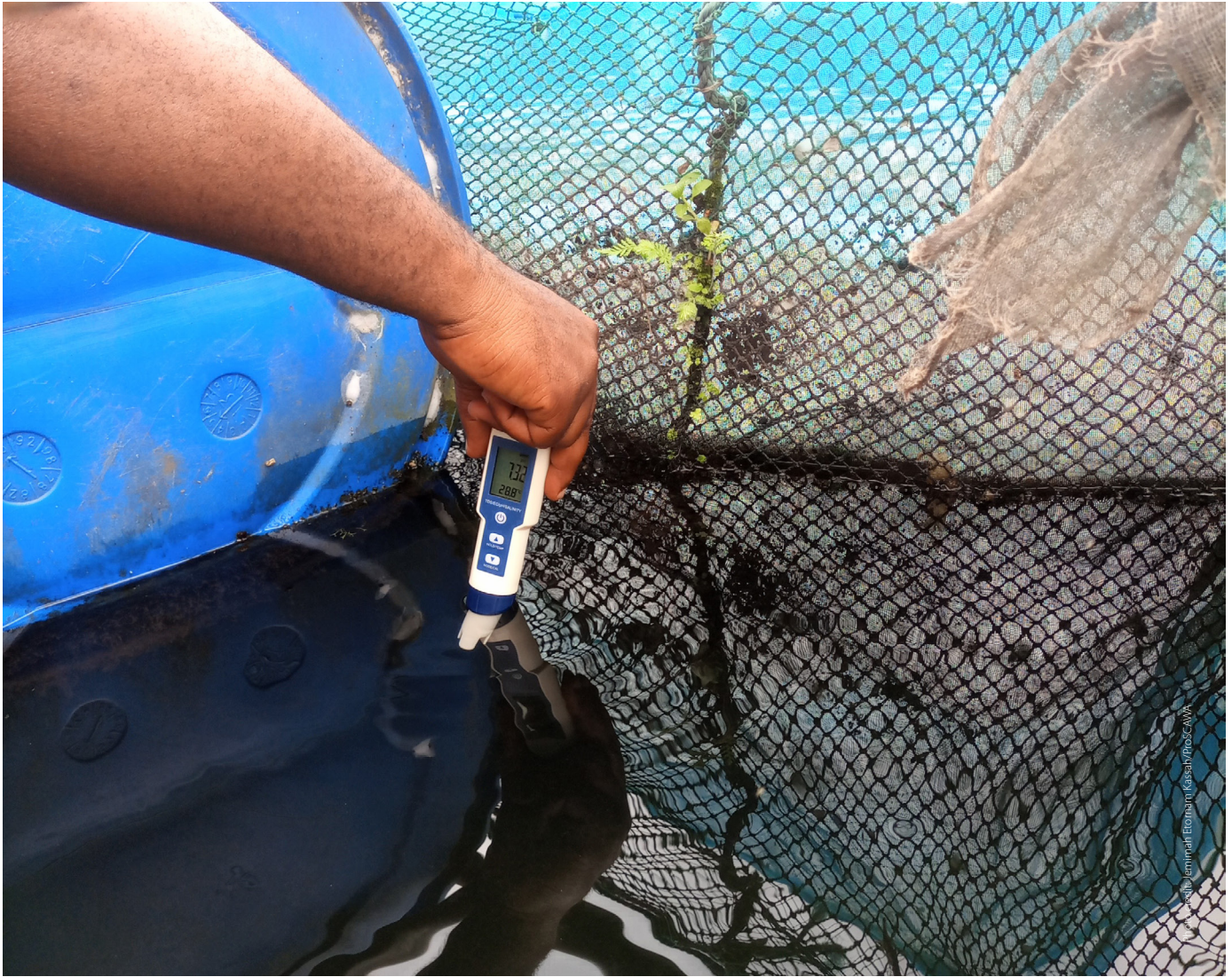
Plate 12. Testing the water quality outside a cage using a portable probe.
